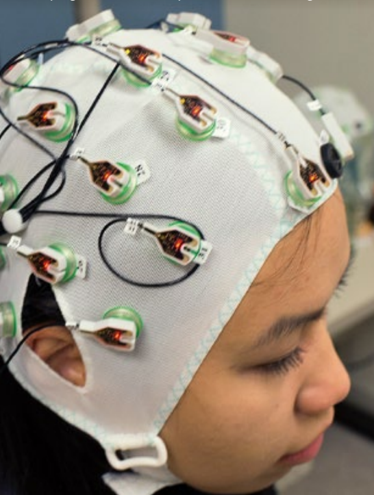
Sensors in a cap allow the Contact Heat Evoked Potential Stimulation computer to detect which parts of the brain react when a patient's extremities are stimulated, helping clinicians detect potential nerve damage.
